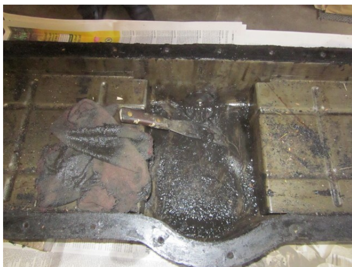
Engine disassembly pieces of piston skirt in the oil pan and cylinders that needed boring.
